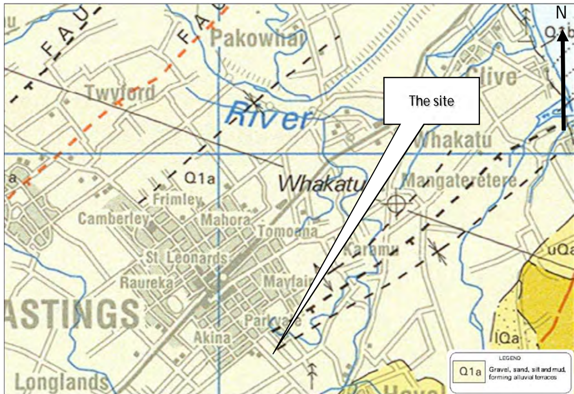
Figure 4.1: Published geology of the site (source: Geology of Hawkes Bay Area , Institute of Geological and Nuclear Sciences)
