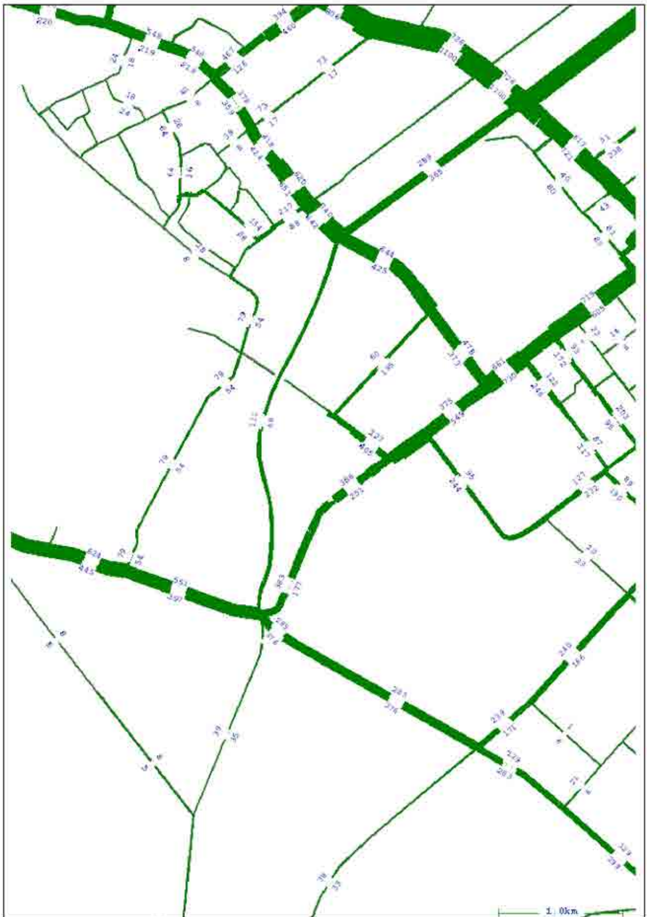
Hawke's Bay Irongate Modelling 2026 AM Peak Irongate with Link Road Stage 2+ Development Traffic Volumes Figure 10 Gabites Porter Consultants
