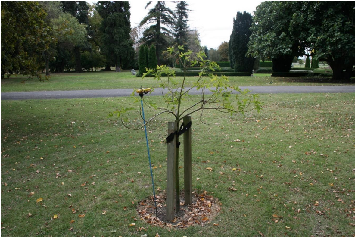
Fig. 10 Illawarra flame tree ( Brachychiton acerifolius ) the root spear is beginning to detect roots at 20cm below ground level.
