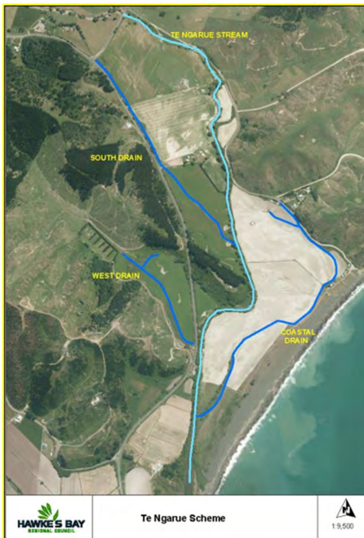
Figure 2.2: Te Ngarue scheme and three private drains
