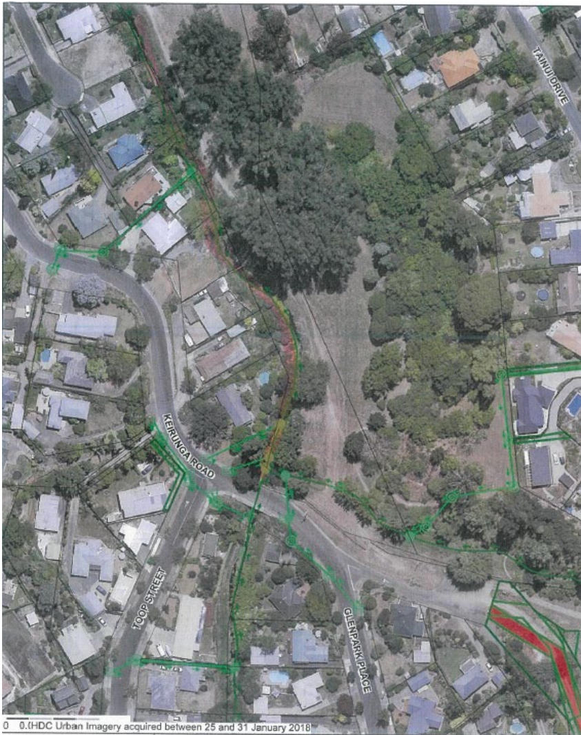
Mangarau Stream (Red denotes Scrub bar, weed Spray and yellow denotes reach mower)
