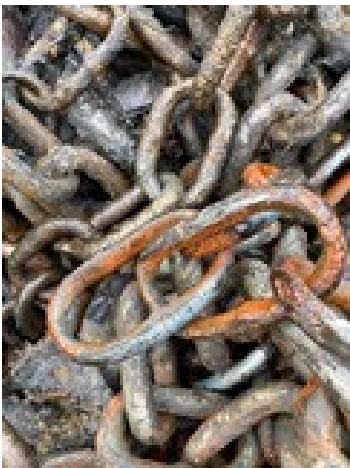
Image 5: Replaced Mooring Chain
