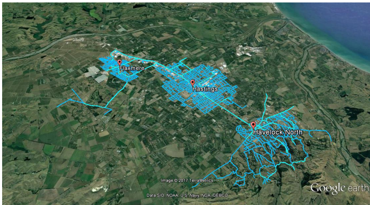
Figure 2.3.1 – Layout of the Hastings Urban Water Supply (excludes Paki Paki)
