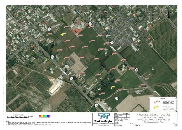
Subsurface conditions encountered during the geotechnical investigations were identified as alluvial deposits, which were considered generally consistent with the geology presented on published geological maps of the area. Up to 400mm of topsoil was encountered, and groundwater was encountered between 1.9m and 4.23m below existing ground levels.
